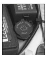
Open the cap labeled WASHER FLUID ONLY. Add washer fluid until the tank is full.
